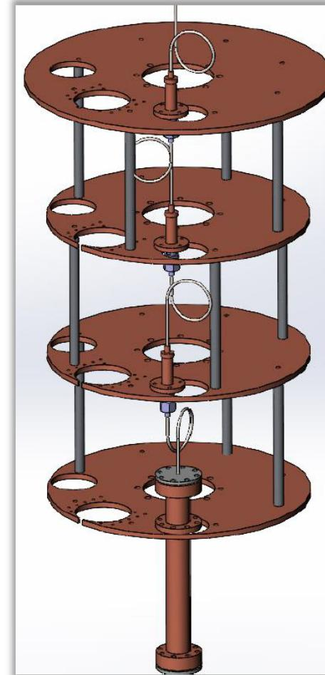
**Purpose:** To test the possibility of (i) generation of various excitations in helium (phonons, rotons, scintillations) by various controlled methods (thermal, mechanical, irradiation with various particles) and (ii) registration of these excitations by microcalorimetric detectors of various types
