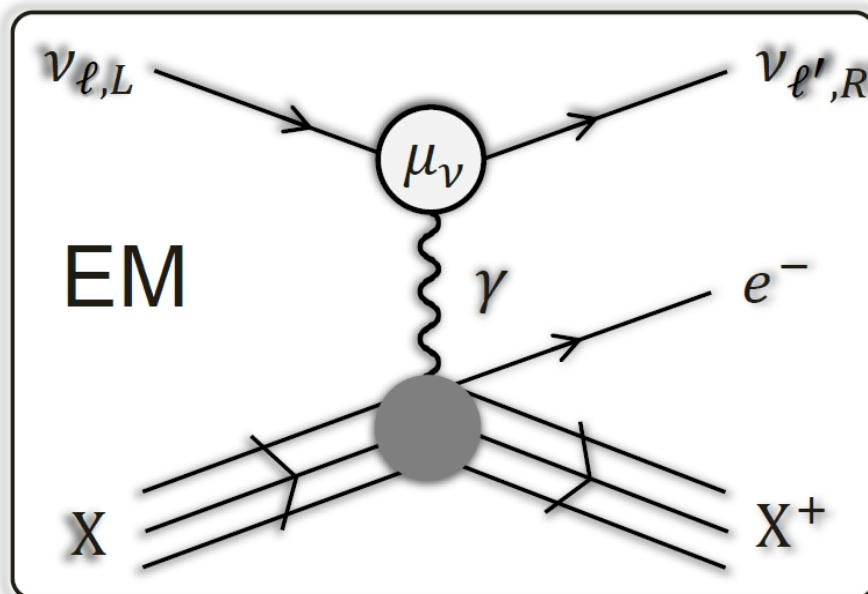
Unlike the SM weak NC and CC interactions, the  $\mu_\nu$  interaction flips the neutrino helicity ( $L \rightarrow R$ ) and can change the neutrino flavor if the transition magnetic moment ( $\ell \neq \ell'$ ) is nonzero.
